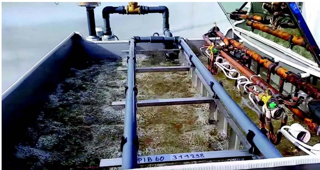
The air pump also stops layering of return water from plate heat exchange, with milk entering the storage vat at 3°C the vat refrigeration will not run until such a time as milk temperature reaches 6°C. With a vat wrap on the vat this could be several hours before main vat unit starts.
